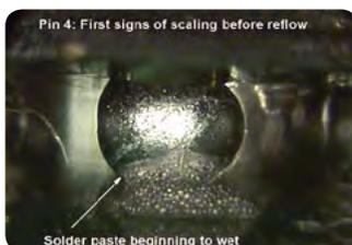
Pin 4: First signs of scaling before reflow
